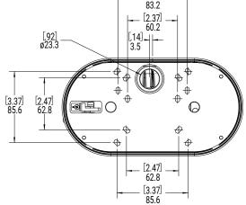
Dual Head Junction Box Mount Camera (H5DH-D1-IR/H5DH-DO1-IR with H5DH-DO-JBOX1 junction box)
